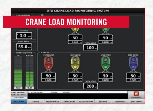
OTD crane load monitoring system is a highly reliable custom-built system for monitoring the load on various cranes and holding platforms in the offshore and marine industry.
