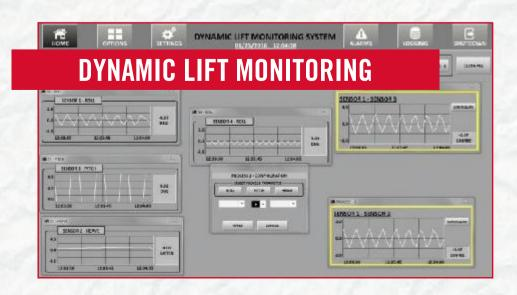
OTD dynamic lift monitoring system is designed for transfer of cargo between ships. The system utilises the latest wireless technology to provide real-time motion information of the primary and target vessels and assist the crane operator in lifting and landing the cargo with reduced load impacts and rope tensions.
