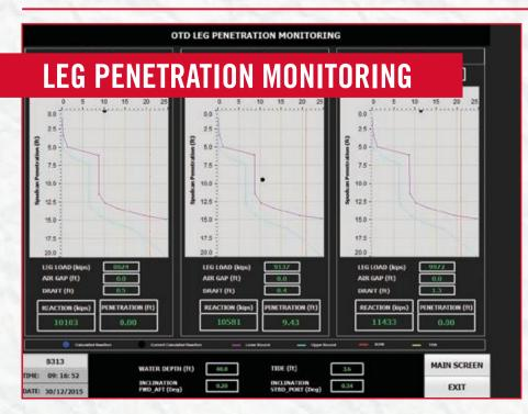
During preloading operation of the jack-up vessel, OTD leg penetration system monitors the leg reaction on each leg against the vessel's penetration curves.
