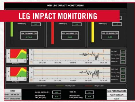
During installation of jack-up vessel, the leg impact monitoring system calculates the distance from leg bottom to seabed for each leg while tracking the motion of the vessel against the allowable limits for the given sea state and environment conditions.
