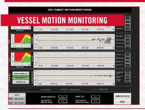
OTD vessel motion monitoring is designed to provide accurate monitoring of the vessel/platform motion during towing operation in the harsh sea environment with real time comparison of vessel motion against the critical design limits.
